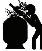
**NEVER** operate the filter system at more than 50 psi of pressure. Operating filter system in excess of 50 psi can cause product failure or also cause the filter lid to be blown off, which can cause death, serious personal injury or property damage.
