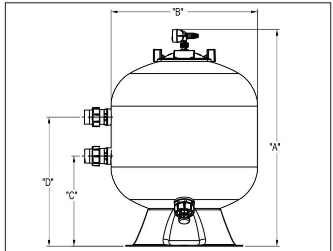
**Figure 1. Jandy JS Series Sand Filters Dimensions**
