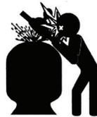
**NEVER** attempt to assemble, disassemble or adjust the filter when there is pressurized air in the system. Starting the pump while there is any pressurized air in the system can cause product failure or also cause the filter lid to be blown off, which can cause death, serious personal injury or property damage.
