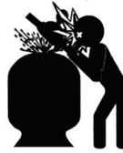
**NEVER** start pump while standing within 5 feet of the filter. Starting the pump while there is pressurized air in the system can cause product failure or also cause the filter lid to be blown off, which can cause death, serious personal injury or property damage.
